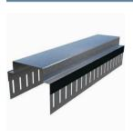
Profile with two slotted lower legs with firestop on both sides. Composite Firestop Deflection Track System with "offset step" accommodates fireproofing up to 1-1/2" thick in head of wall and wall to wall (column) assemblies. Two legs with slots spaced 1" o.c. for positive attachment of studs.
