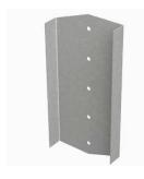
EasyClip™ QuickTwist™ web stiffeners are used to provide reinforcement of joist webs to prevent crippling. Web reinforcement is often required by design to enhance the load capacity of joists. The unique design of QuickTwist allows the installer to insert the stiffener on the inside of the joist after the joist is installed. This stiffener eliminates the need to pre-insert traditional web stiffeners prior to joist installation. The one-piece assembly is easily rotated in place for a tight fit.
