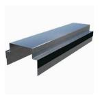
Profile with two solid legs with firestop on both sides. Composite Firestop Deflection Track System with "offset step" accommodates fireproofing up to 1-1/2" thick in head of wall and wall to wall (column) assemblies.
