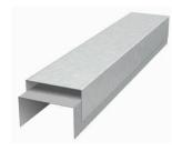
ClarkDietrich DoubleTrack™ system is a two-piece assembly that accommodates deflection of exterior curtain walls. A custommade deep leg outer track is installed to the underside of the floor deck. A wall assembly is constructed on the floor and slid into place, with a "gap" at the top for deflection. DoubleTrack deflection assemblies cannot be used in axial load-bearing stud conditions or above continuous window spandrels.
