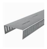
MaxTrak 2D is a head-of-wall deflection track that is used for framing exterior curtain walls and nonload-bearing interior walls where vertical deflection and horizontal drift occurs—and serves as a connecting member that isolates the cold-formed steel framing system from the movement of the primary structure.
