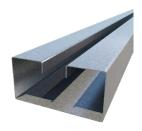
This HDS header stud is precut to the length specified length on your order. The system provides cost-effective, member-reducing framing solutions. Header lengths should be ordered 1/2" shorter to fit inside clips. All material CP60.
