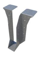
Bridle hangers are commonly used to attach cold-formed C-joists to structural steel beams, wood ledgers or masonry block. Connections can be made with screws, powder-actuated fasteners, drill-in concrete anchors or welding. Single- and double-wide hangers are also available in other widths and depths. The MB hanger can also be sloped to a maximum of 45°. Skew only: MB series can be skewed to a maximum of 45°maximum allowable download is 62% of table load.
