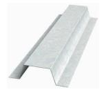
ClarkDietrich heavy-duty furring channel is a high-performance framing component used in ceiling, exterior wall and roof applications. With two standard depths—7/8" and 1-1/2"—heavy-duty furring channel provides greater resistance to deflection and bending. In roof applications, heavy-duty furring is used as purlins to provide connection points for roof sheathing.
