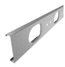
ClarkDietrich TradeReady® steel joists meets the requirements of most typical building layout and floor/roof loads. Large extruded holes (spaced at 24" o.c.) accommodate HVAC, mechanical, plumbing, electrical and sprinkler runs. The joist also features a series of smaller holes for electrical and technology lines. Hole sizes range from 4-1/4" oval to 10" round, based on member depth.
