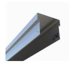
The BlazeFrame RipTRAK is the only UL tested fire-rated head of wall joint system that offers an alternate listing by eliminating castle cuts and sealant. Meets UL 2079, 5th edition; HW-D-1125 and HW-D-0823. For alternate details, please refer to configuration A, items 3A1 and 3B1. This is good for both roof and wall assemblies.
