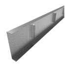
Another major component of the TradeReady floor system, the standard 12'-long rim drastically reduces framing time and effort. Rims have pre-formed, prepunched attachment tabs at 12", 16", 19.2" or 24" o.c. spacing to eliminate layout time-and ensure fast, proper fastener placement. Embossed stiffening ribs on each side of the tabs provide additional reinforcement, for a significant reduction of web stiffeners (squash blocks) and support clips in a majority of applications.
