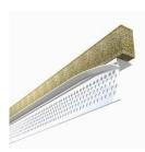
Vinyl L-Bead with compressible foam. UltraBEAD, when used in conjunction with UltraTRAK slotted deflection track or Deep Leg deflection tracks, provides joint protection up to ¾" for a 1 or 2 HR concrete deck Head of Wall Joint System at 60% compression.
