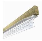
Vinyl L-Bead with compressible foam. UltraBEAD, when used in conjunction with UltraTRAK slotted deflection track or Deep Leg deflection tracks, provides joint protection up to ¾" for a 1 or 2 HR concrete deck Head of Wall Joint System at 60% compression.
