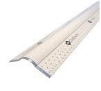
Off-angle nail-on bullnose bead, also known as splayed bullnose or 120°/135° bullnose corner bead, is used to provide a rounded bullnose finish for outside off-angle drywall intersections. Nails or mechanical fasteners are used to secure the bead to the wallboard.
