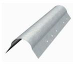
Bullnose corner bead is used to create a smooth, rounded look to standard drywall corners. Bullnose adds contemporary styling and a sense of openness to any room. Bullnose bead is nailed, screwed or stapled in place and finished with joint compound. Bullnose is available with a galvanized finish meeting ASTM C1047 standard.
