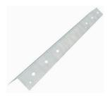
Clinch-On hot-dipped corner bead offers the identical roll-formed precision as its counterpart. Hot-dipped galvanized metal corner bead (meets ASTM C1047) provides enhanced corrosion protection and reinforcement at exposed 90° corners. Flanges are knurled and perforated to ease joint compound adhesion and nail attachment.
