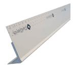
L-trims are used to finish the ends of wallboard where it abuts dissimilar surfaces, such as suspended ceilings, beams, plaster, masonry or untrimmed door and window jambs. Applied in the same manner as all other tape-on beads-joint compound embeds the paper-faced bead to the wallboard paper.
